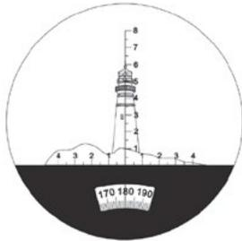
**Example:** The object height of the pictured lighthouse is 60 m. For the height of the lighthouse, the value 6.0 can be read on the graticule.
